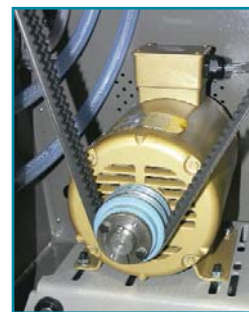
NEMA Premium® efficient inverter-driven motor
